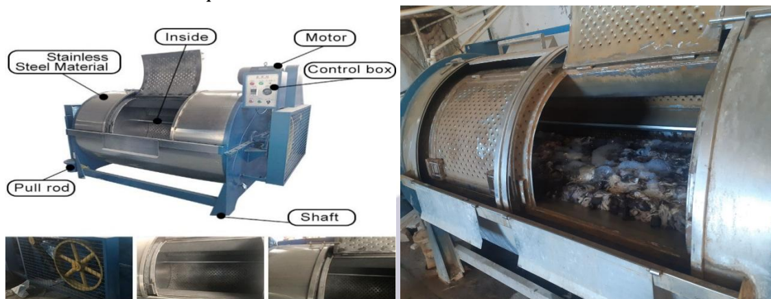
6-rasm. Zamonaviy intensiv yuvish jihozi
