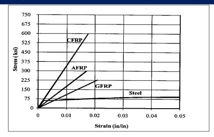
Rice. 1.2. Stress-Strain Relationship for FPM: Carbon Fiber (CFRP), Glass Fiber (GFRP), Aramido-Fibrous (AFRP) and Steels
