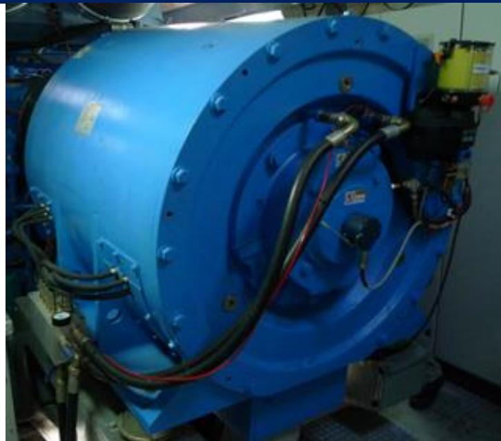
**Highly-reliable wind turbine technology. Hermetically-closed permanent magnet synchronous generator (PMSG) achieving an increased power generating efficiency with no need of external excitation system**
