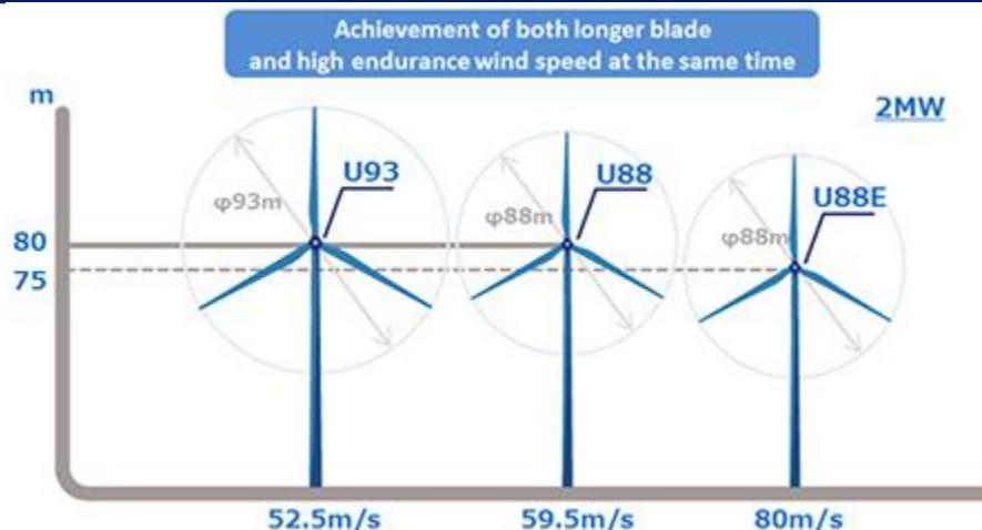
We have variety of WTGs with long blades that covers wide range of endurance wind speed, and so we are able to provide WTGs that are suitable for each site. We also keep developing large WTGs for onshore/offshore in order to decrease the unit cost.
