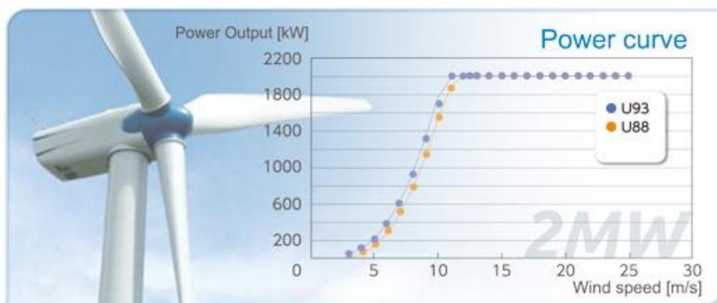
\* IEC standard: Reference wind speed 50 m/s, average wind speed 8.5 m/s, extreme wind speed ( $V_{e50}$ ) 70 m/s.
