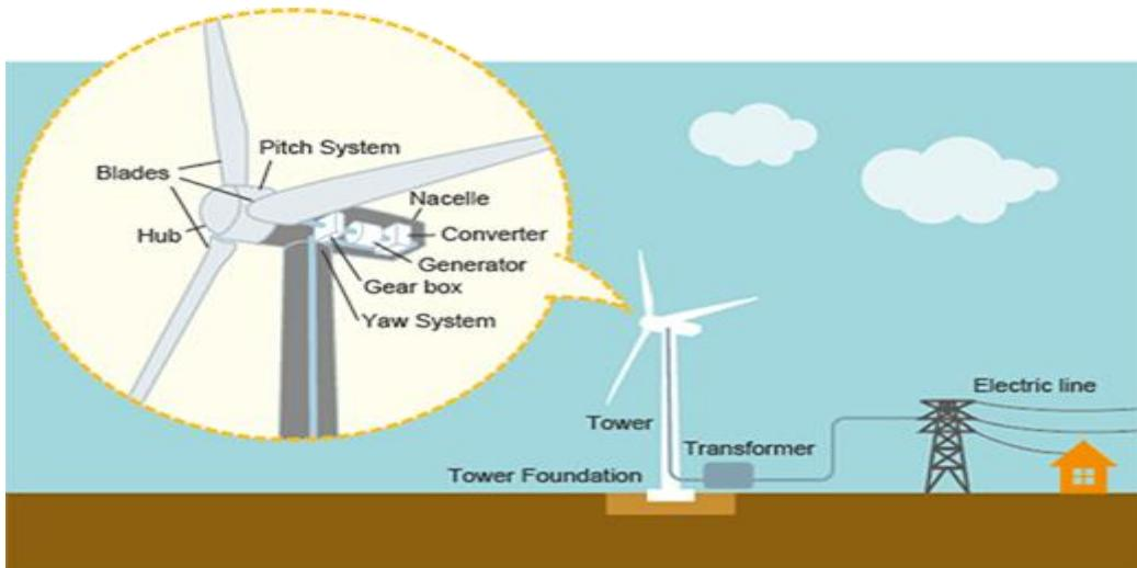
Introduction of wind power generation has been increasing in the world, which has the following characteristics:
