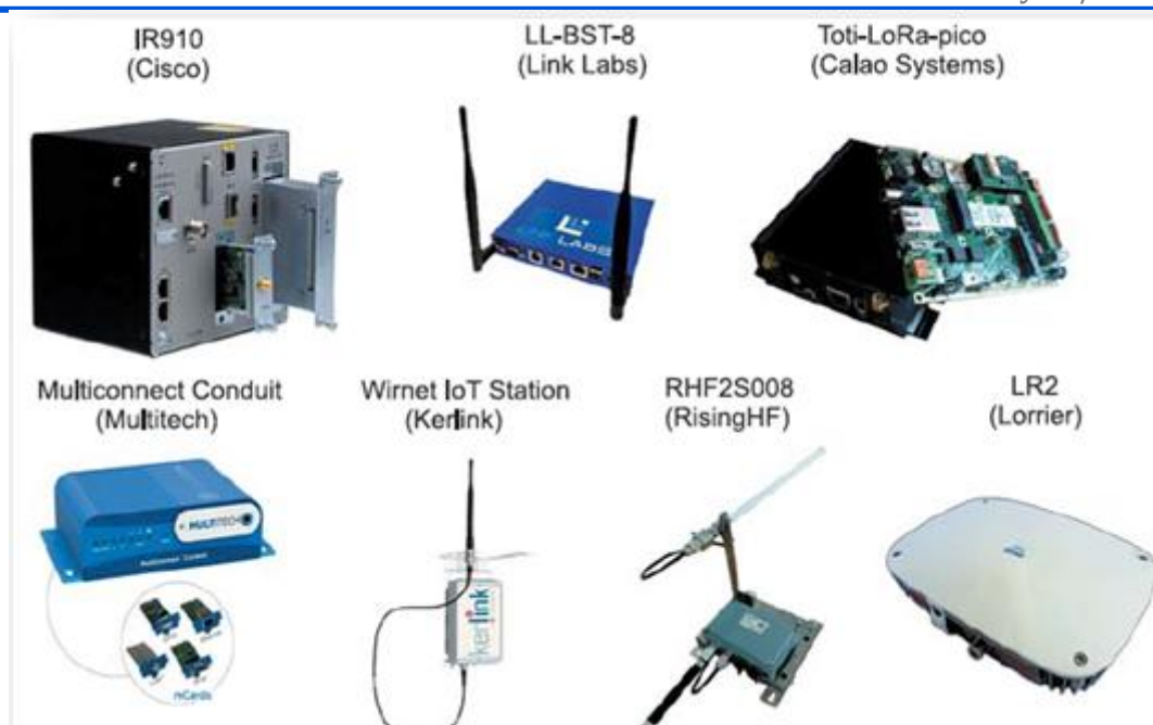
5-rasm. LoRaWan alohida bazaviy stansiyalarining tashqi ko‘rinishi
